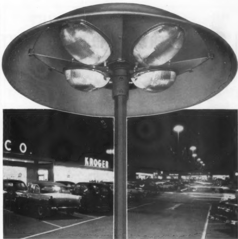
New No. 5442 Ultra-Lite. Four mercury luminaires are tilted 15° for improved high level, uniform light distribution. Lamps and Alzak aluminum reflectors are housed under modern parabolic dome of spun aluminum.
